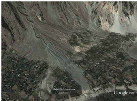
Figure 26 — Typical geomorphological features of mud flows of various ages on an alluvial fan Hatoon, Khizer District, Pakistan, 36°16' N, 73°45' E (Google Earth, accessed March 2013)
