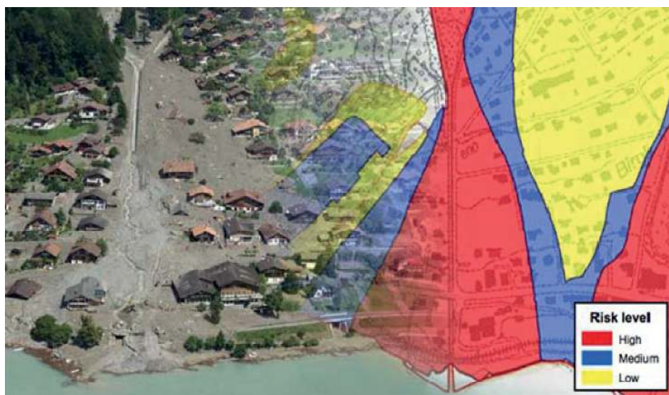
Figure 1 — Flooded area (mud flow) and simplified risk map for an Alpine town in Switzerland
