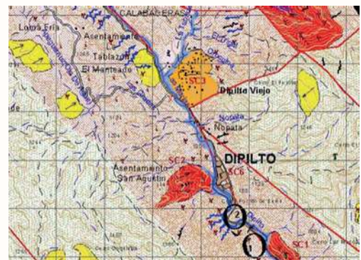
Figure 18 — Hazard zoning indication map on landslides and flooding with Swiss system applied in Nicaragua (República de Nicaragua, Municipio de Dipilto). SDC’s disaster reduction programme for Central America, Managua, 2003 in SDC, 2005
