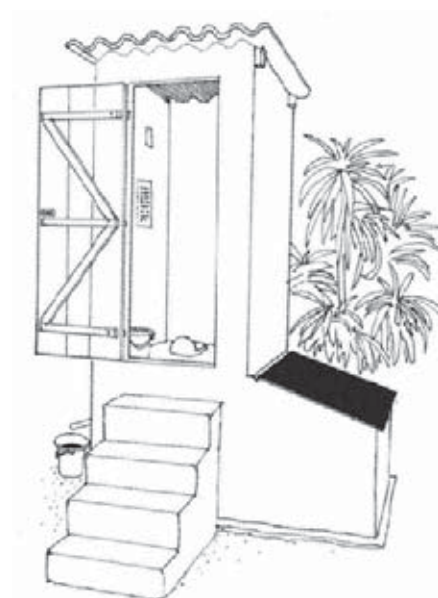
UDDT with solar heated composting chamber - Vietnam
